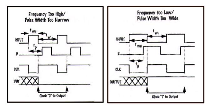
When it is required to detect a clock frequency that exceeds a certain value, this effect can be eliminated by a slight circuit modification: inverting the input signal to provide clock for the flip-flop and feeding the D input with the delayed input clock. (See *Detecting Clock Frequency Above Limit* diagram.) In this configuration, the maximum limit on clock frequency is reached when the input pulse width,  $t_{WH}$  or  $t_{WL}$ , becomes equal to the individual delay element value  $t_D$ .
